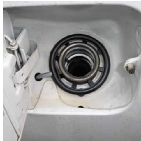
Ring Antenna installed over filler neck.
