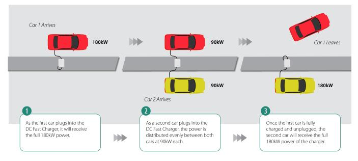
Featuring optional liquid cooled cables, the 180kW AiO DC Fast Charger can provide an 80% EV battery charge in as little as 10 to 15 minutes, offering the capability to serve more customers in less time.
