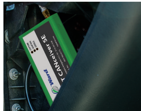
CANceiver installed under dashboard
